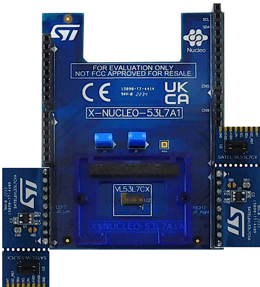
Figure 7. SATEL-VL53L7CX breakout boards connected to the X-NUCLEO-53L7A1 expansion board
